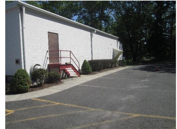
Parking spots south of the building can be replaced with porous asphalt to capture and infiltrate stormwater. Downspouts along the building can be disconnected and directed into porous asphalt parking spaces in order to decrease runoff. A preliminary soil assessment suggests that more soil testing would be required before determining the soil's suitability for green infrastructure.
