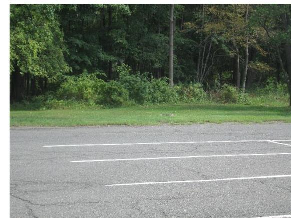
Parking spots east of the building can be replaced with porous asphalt to capture and infiltrate stormwater. A rain garden can be built adjacent to the parking lot to capture, treat, and infiltrate runoff. A preliminary soil assessment suggests that more soil testing would be required before determining the soil's suitability for green infrastructure.
