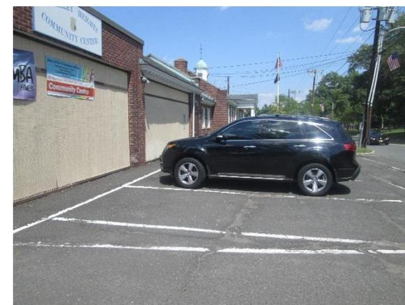
Parking spots adjacent to the building can be replaced with porous asphalt to capture and infiltrate stormwater. Also a downspout by the southern parking lot can be directed into the porous asphalt parking spaces in order to decrease stormwater runoff. A rain garden can be built to capture, treat, and infiltrate roof runoff. A preliminary soil assessment suggests that more soil testing would be required before determining the soil's suitability for green infrastructure.
