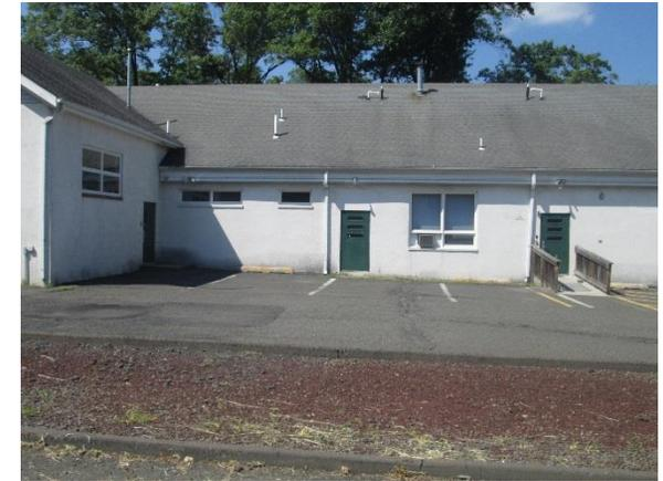
Parking spots adjacent to the building can be replaced with porous asphalt to capture and infiltrate stormwater. Downspouts along the building can be disconnected and directed into porous asphalt parking spaces in order to decrease runoff. A preliminary soil assessment suggests that more soil testing would be required before determining the soil's suitability for green infrastructure.
