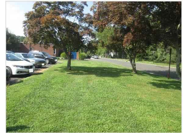
Parking spots to the east and west of the building can be replaced with porous asphalt to capture and infiltrate stormwater. Installing a rain garden adjacent to the building can capture, treat, and infiltrate roof runoff. A preliminary soil assessment suggests that the soils have suitable drainage characteristics for green infrastructure.
